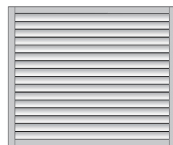
HORIZONTAL LOUVRE INFILL 58MM, 80MM OR 120MM
