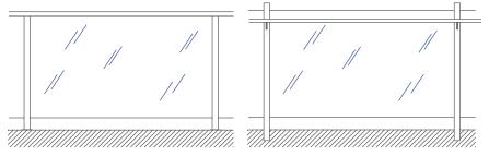
GLASS WITH HANDRAIL (TOP MOUNTED). TOP FIX
